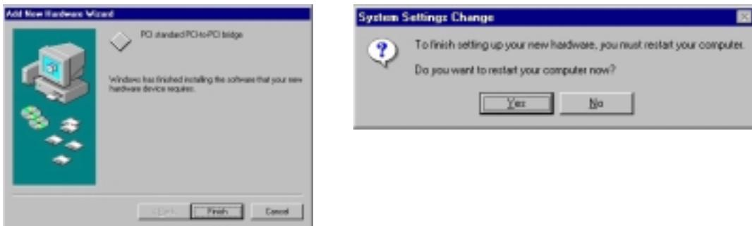
Finally, to ensure the Product is being installed properly, please go to the **Device Manager** of Properties in **My Computer** and double-click **1394 Bus Controller** and **Universal Serial Bus controllers** area, the **PCI OHCI Compliant IEEE 1394 Host Controller** and **Lucent USB Open Host Controller** are being shown respectively and no Yellow! Or red X mark in front of them. It verifies the Product is being installed correctly.
