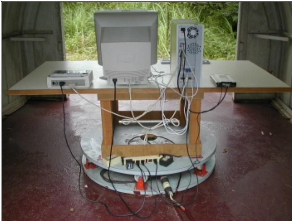
Radiated Emission Setup Photos (Worst Emission Position)
