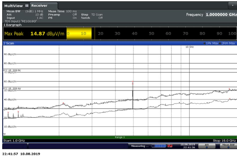
Note: Radiated spurious emissions measurements were performed from 30 MHz to 25 GHz.
