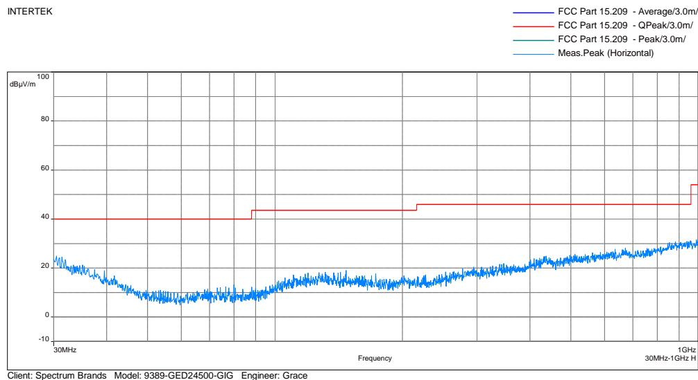
**Radiated Spurious Emissions, 30 MHz – 1 GHz, High Channel, Vertical**
