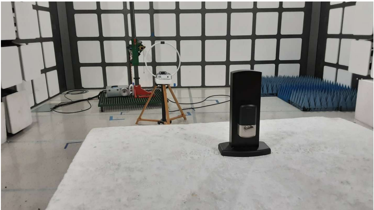
Below 30MHz Emission Set-Up
