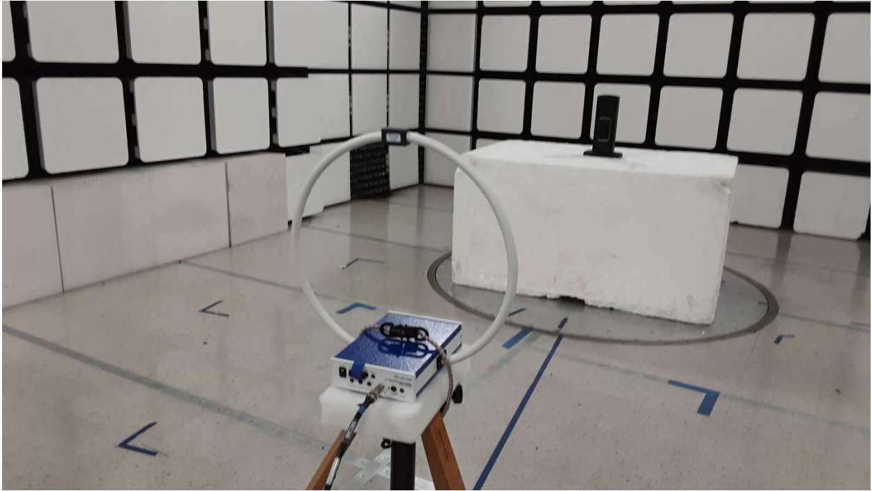
Below 30MHz Emission Set-Up
