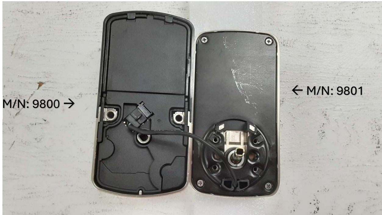
Model: 9801 Back View showing the cable to the model: 9800
