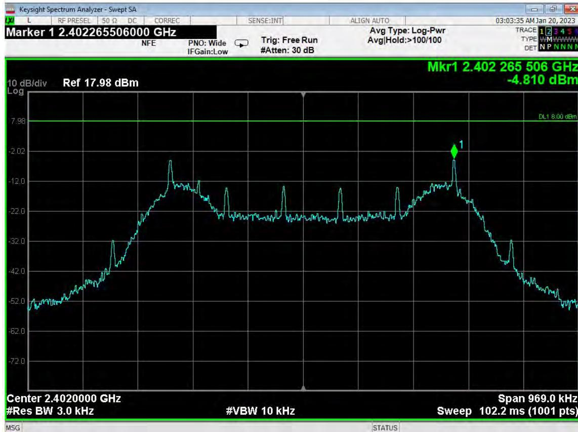
Spectral Density Output - 2402 MHz - -4.810 dBm
