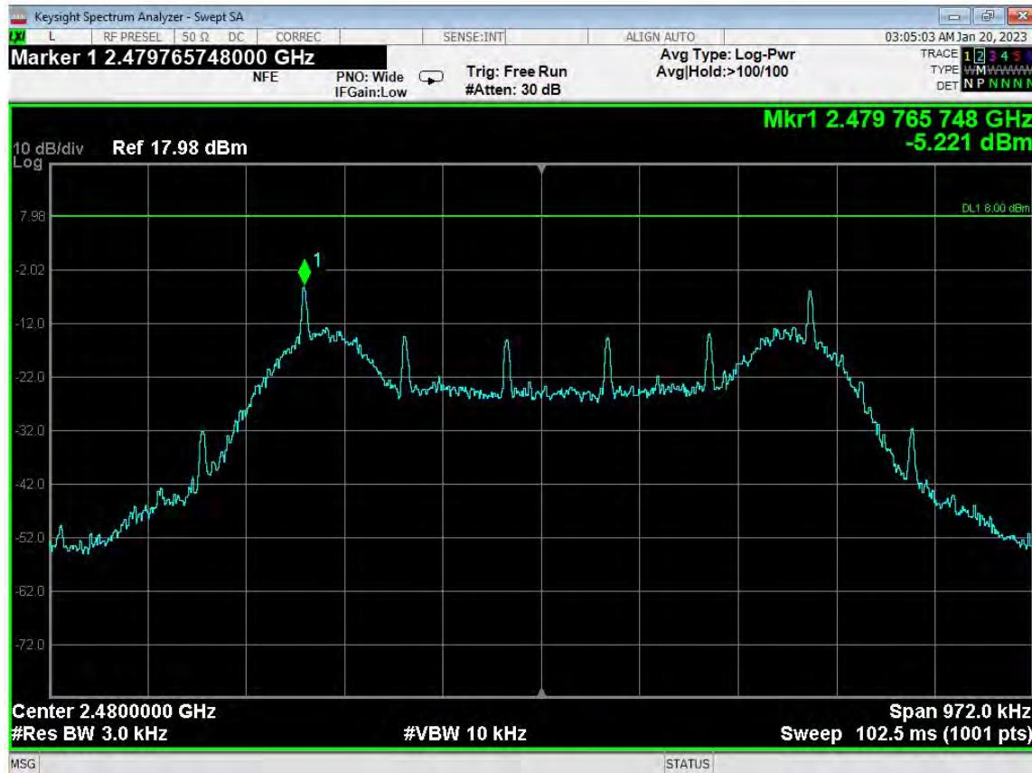
Spectral Density Output - 2480 MHz - -5.221 dBm
