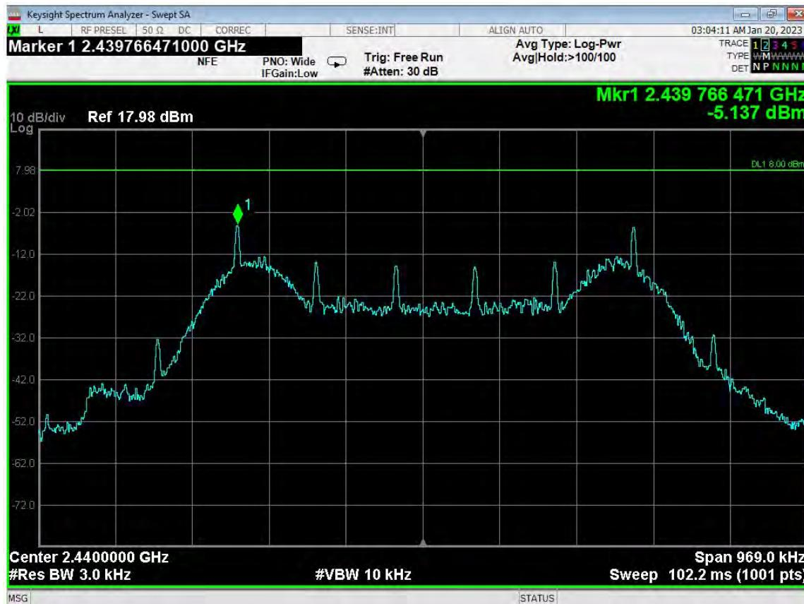
Spectral Density Output - 2440 MHz - -5.137 dBm
