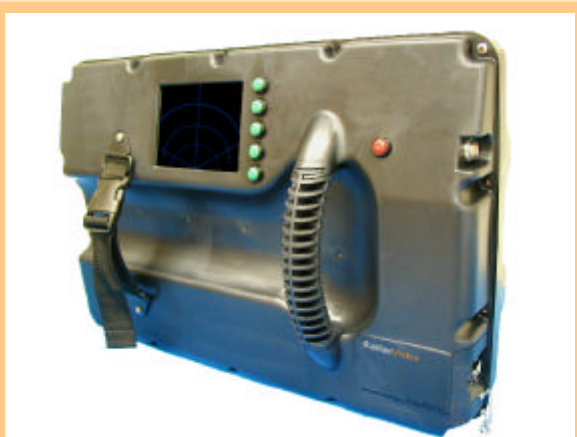
RadarVision: the hand-held ultra wideband device that enables users to detect the movement of people behind walls
