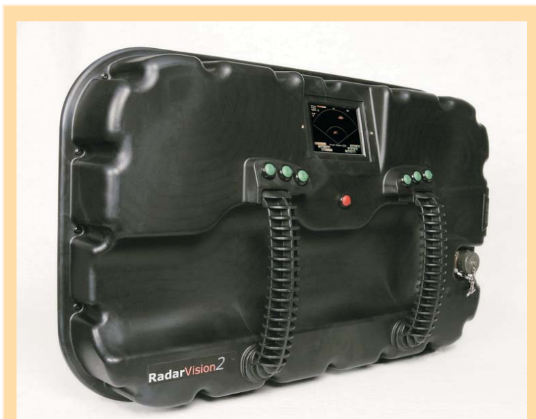
RadarVision2, the second generation hand-held radar device enables users to detect the movement of people behind walls
