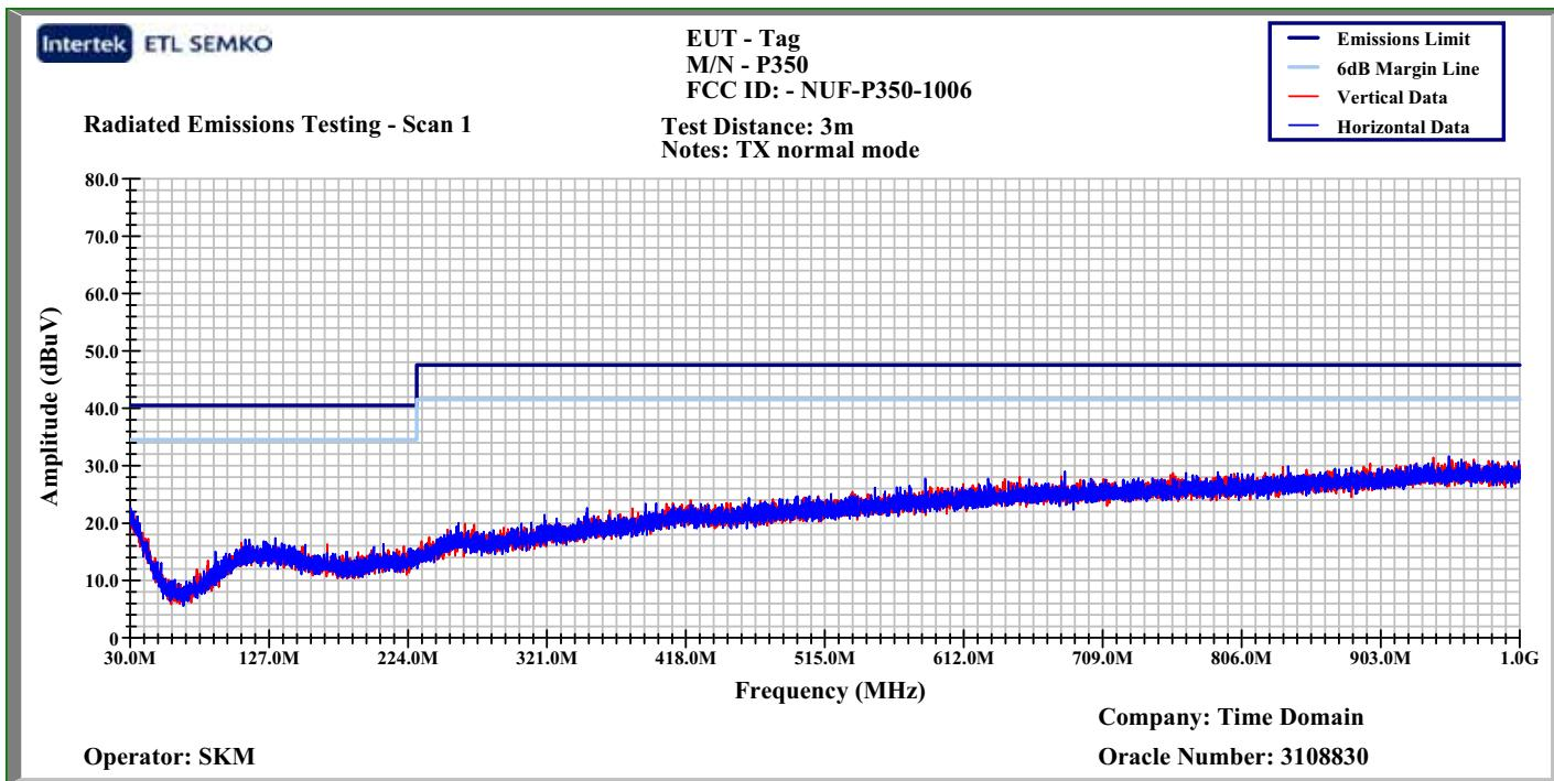
**9.0 15.250(d)(2) Radiated power (EIRP) density in GPS receive bands (EIRP power density (GPS))****Method:**
