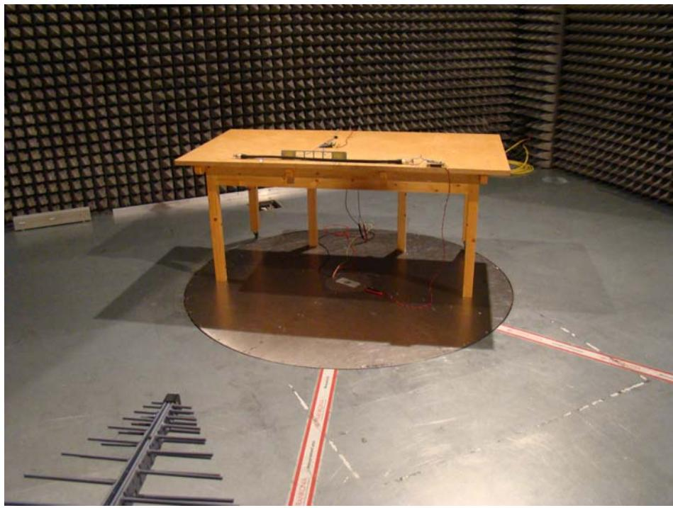
**Test Setup conducted measurements**
