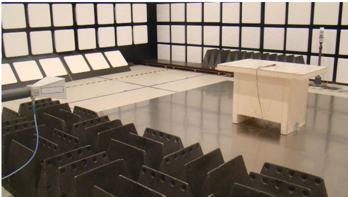
Figure 3: Test setup for Radiated Emission – Above 1GHz (Vertical)
