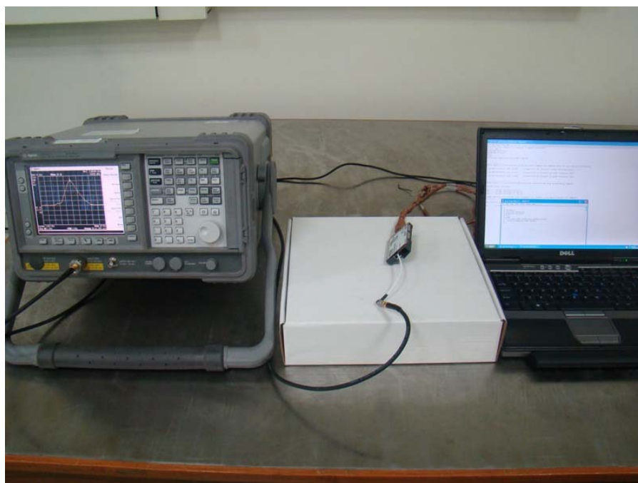
Figure 5: Test setup for Conducted Radio Frequency measurements
