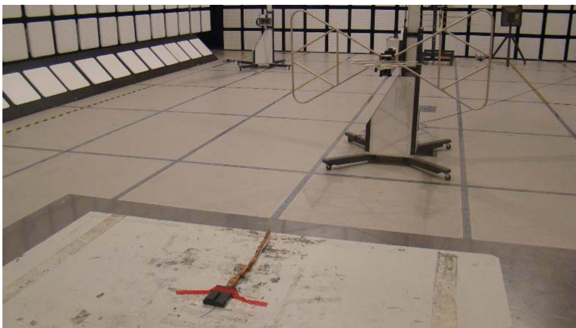
Figure 2: Test setup for Radiated Emission (Horizontal) – 30MHz to 1GHz
