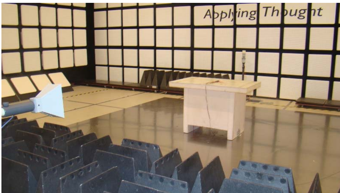
Figure 4: Test setup for Radiated Emission – Above 1GHz (Horizontal)
