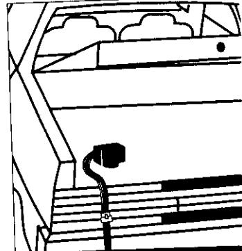
To recharge la Wireless Tow-Light Bar, simply use the standard 12V/110V recharging unit that is included in your package. Plug the adapter into any 110 outlet, and the adapters plug into the right side of the Wireless Tow-Light Bar. The battery will be fully charged in four hours.
