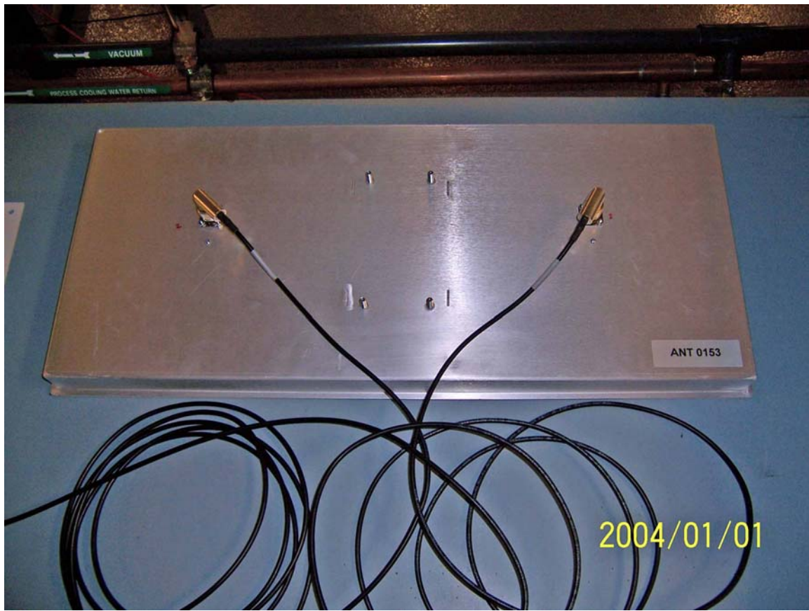
Panel antenna connector side
