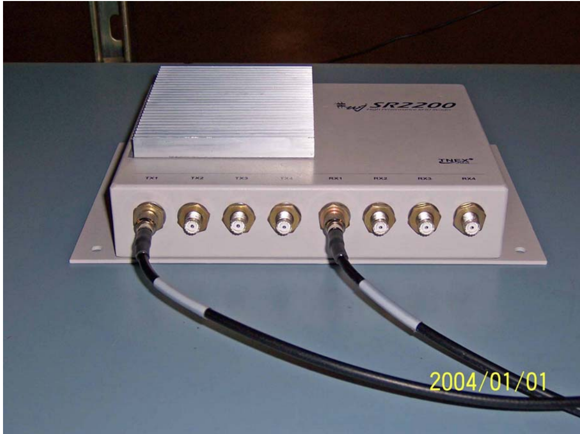
TX and RX antenna ports
