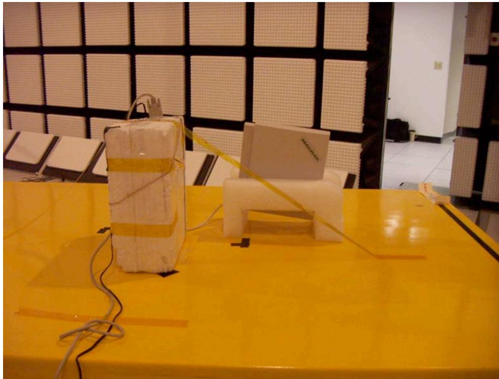
**RADIATED RF MEASUREMENT SETUP (X ORIENTATION)**
