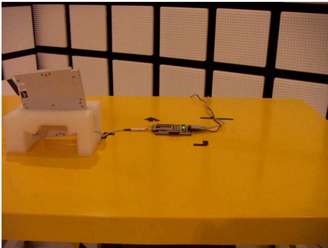
**RADIATED RF MEASUREMENT SETUP WORST CASE (Y ORIENTATION)**
