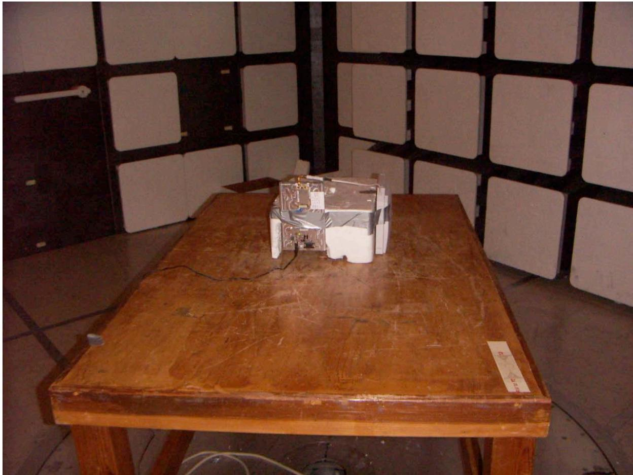
**RADIATED RF MEASUREMENT SETUP ON OATS**
