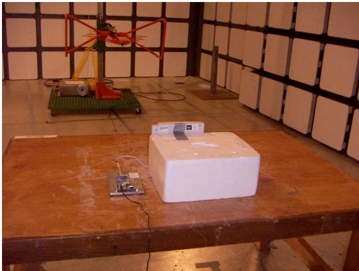
**RADIATED RF MEASUREMENT SETUP (Z ORIENTATION)**
