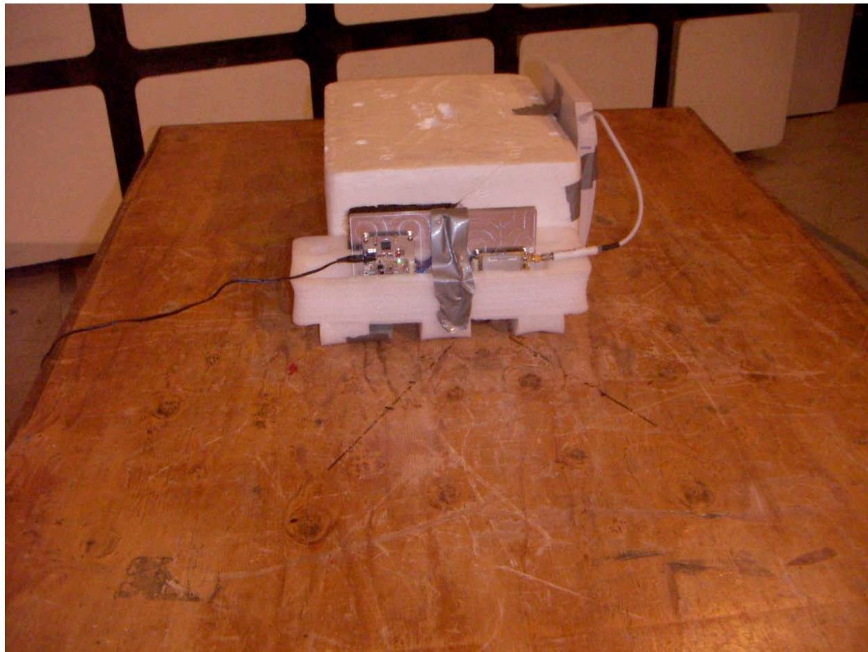
**RADIATED RF MEASUREMENT SETUP (X ORIENTATION)**
