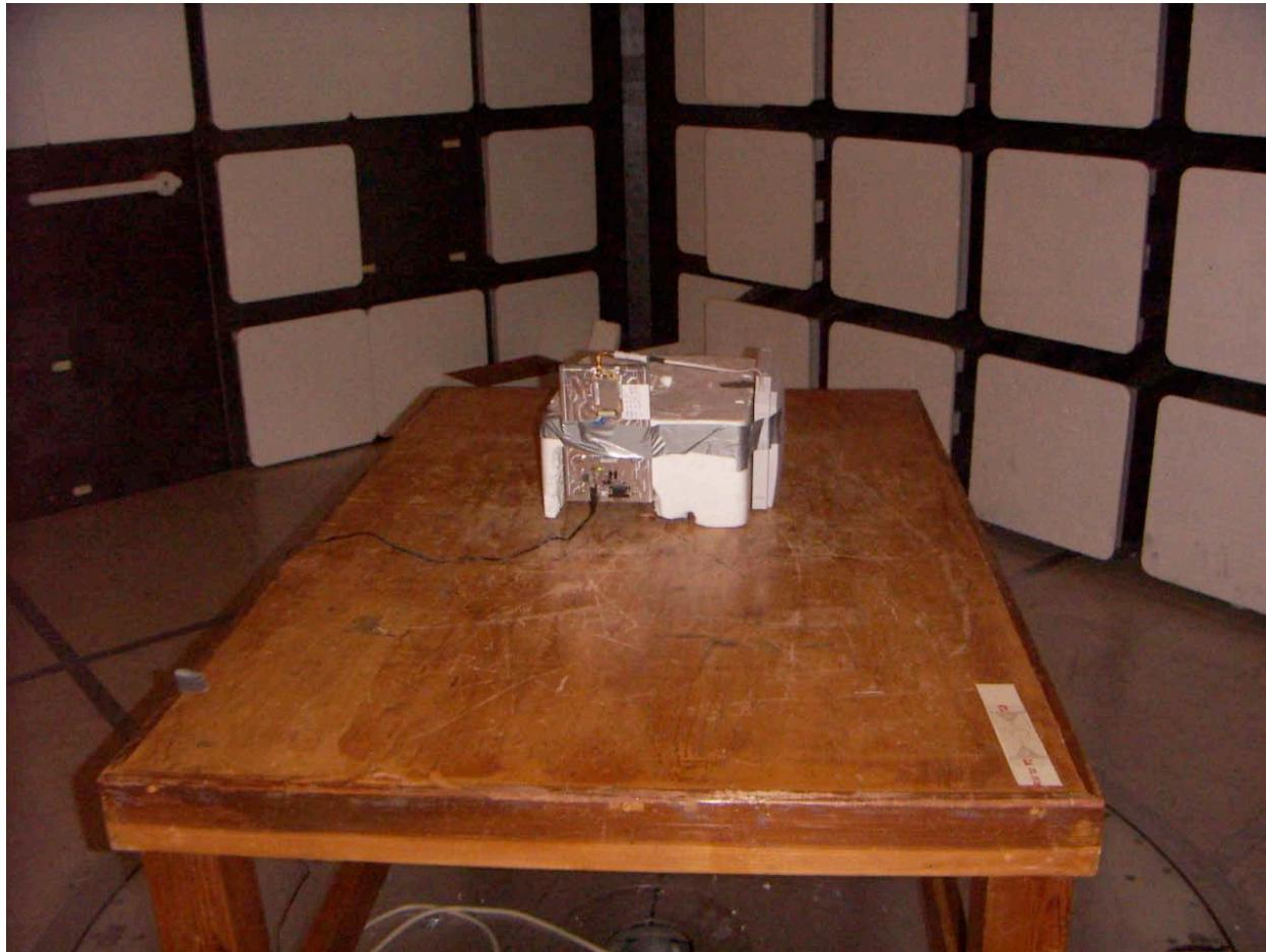
**RADIATED RF MEASUREMENT SETUP ON OATS**
