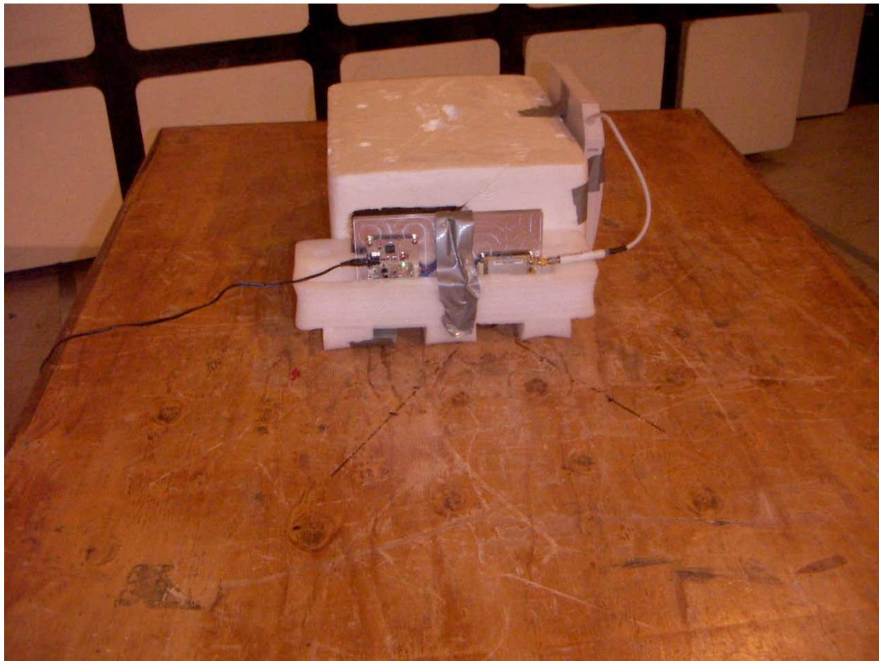
**RADIATED RF MEASUREMENT SETUP (X ORIENTATION)**
