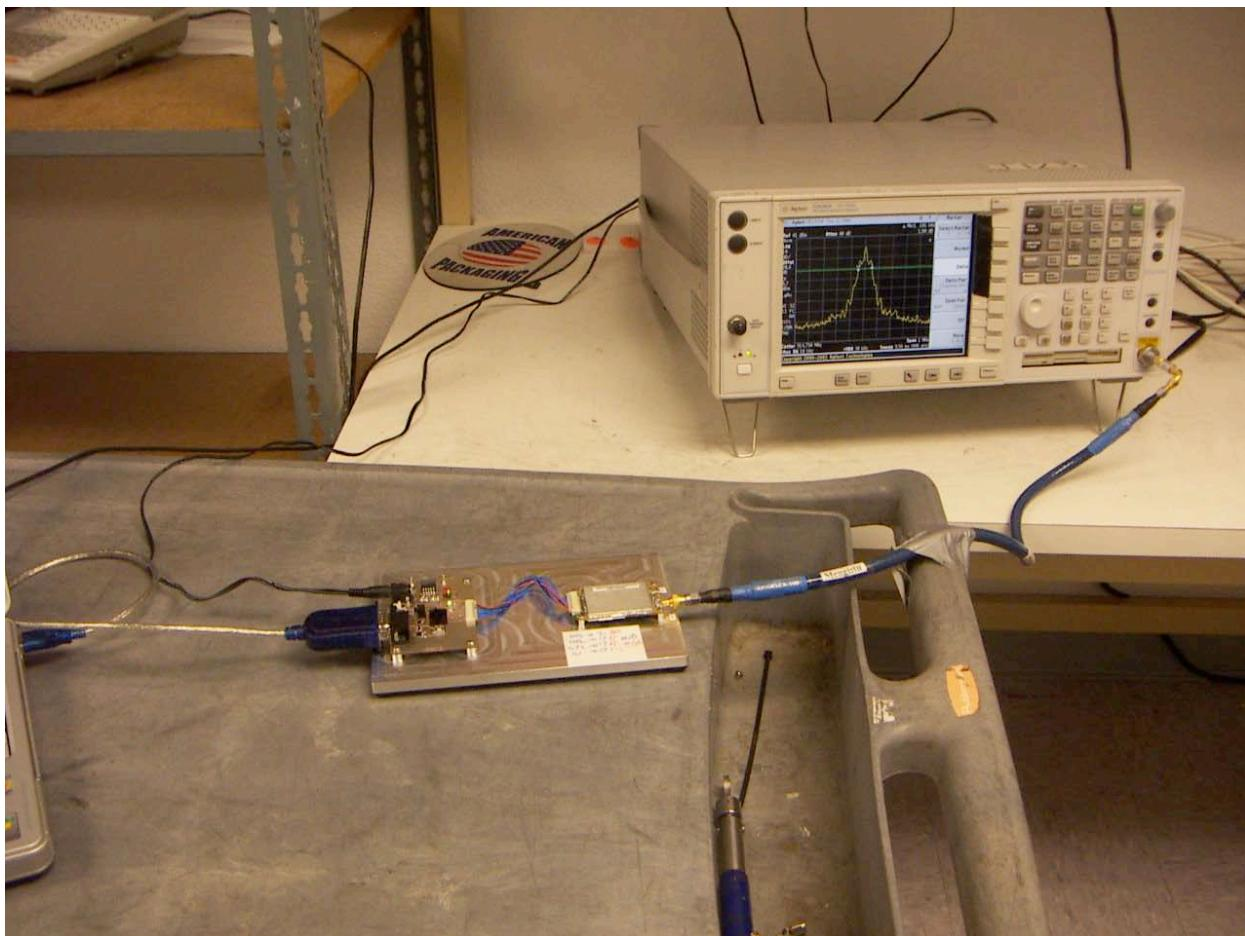
**RADIATED RF MEASUREMENT SETUP (Y ORIENTATION, WORST CASE)**
