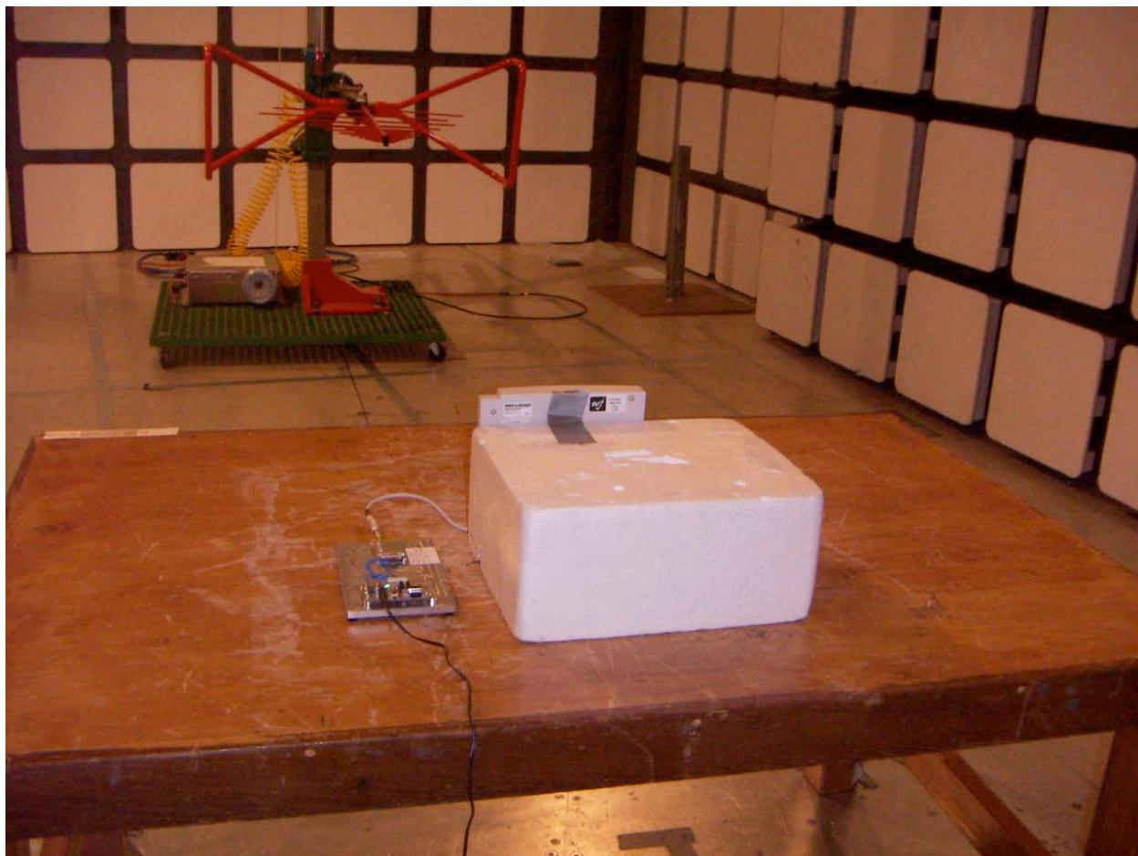
**RADIATED RF MEASUREMENT SETUP (Z ORIENTATION)**
