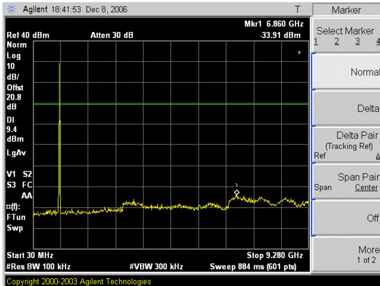
**SPURIOUS EMISSIONS, HIGH CHANNEL (Worst Case Modulation SRE02)**
