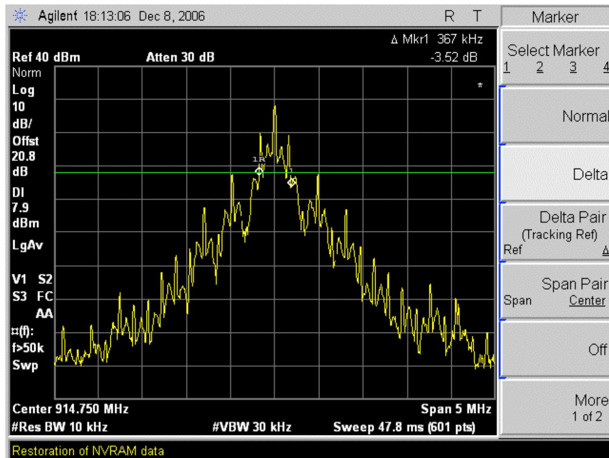
**20 dB BANDWIDTH HIGH CHANNEL (Worst Case Modulation: SRE0)**
