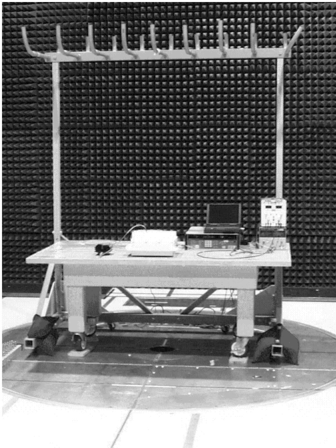
**Case Radiated Test Equipment**
