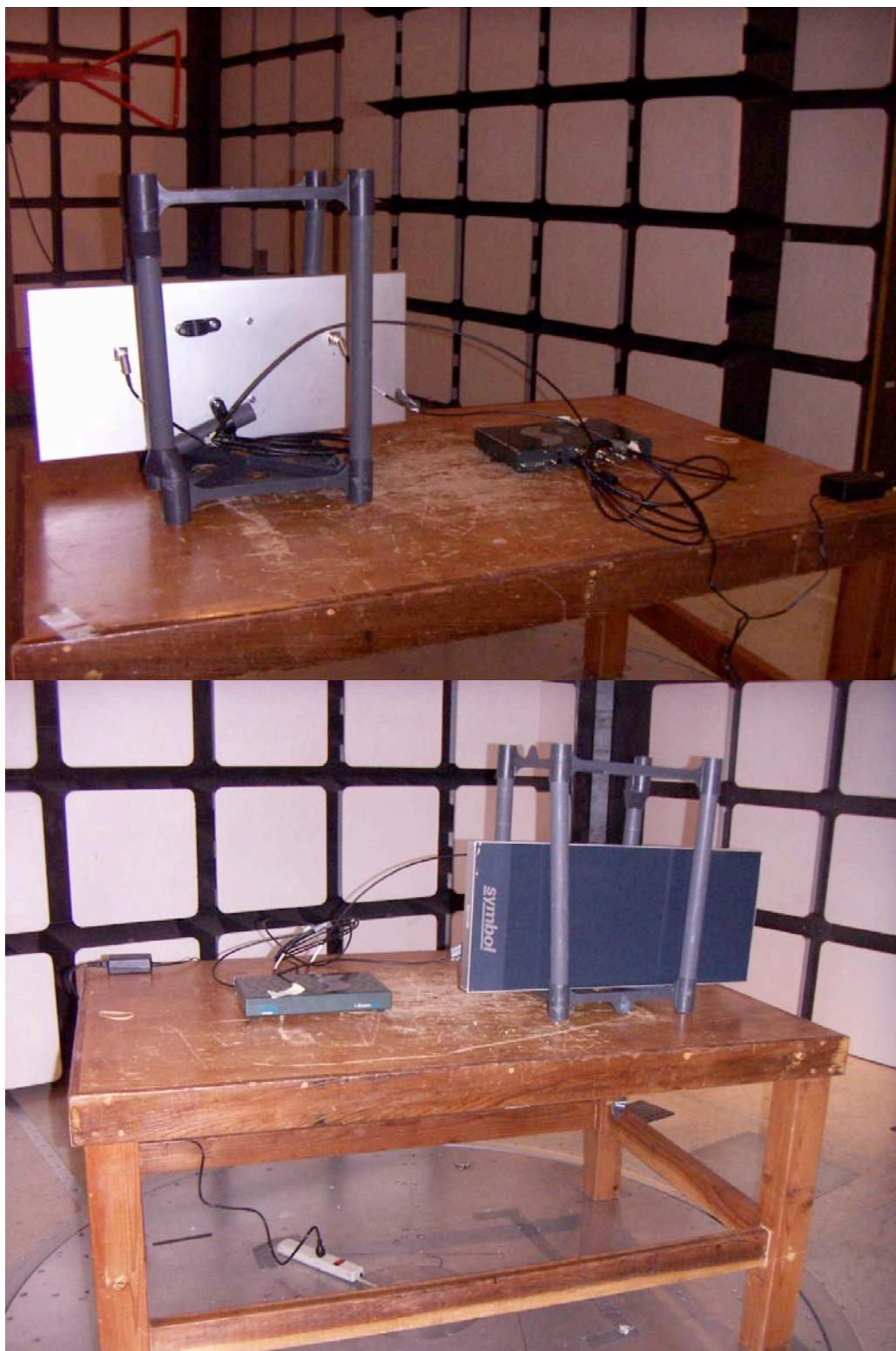
**POWERLINE CONDUCTED EMISSIONS MEASUREMENT SETUP**
