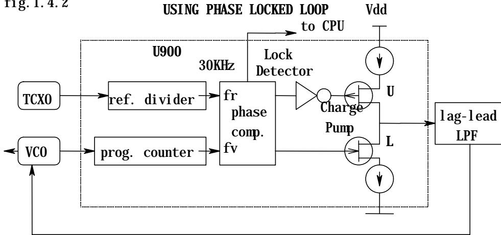
As the output of charge pump gives pulse wave, the second order lag-lead low pass filter is used to generate smooth waveform for VCO control.
