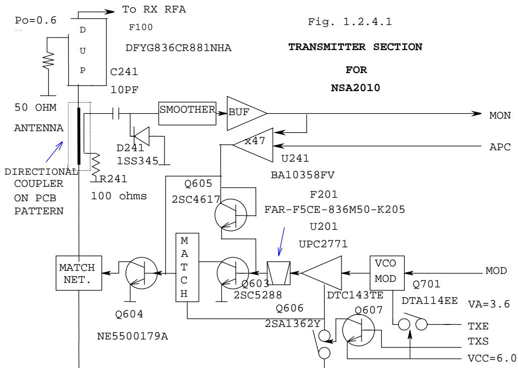
The modulated FM signal generated by TX VCO is amplified by U201 and obtained about 10mW (10dBm) output power on U201.
