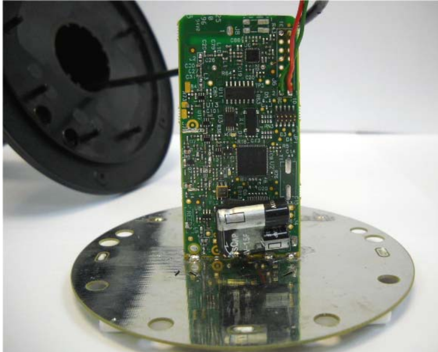
Photograph No.3 2WB-LG booster internal view
