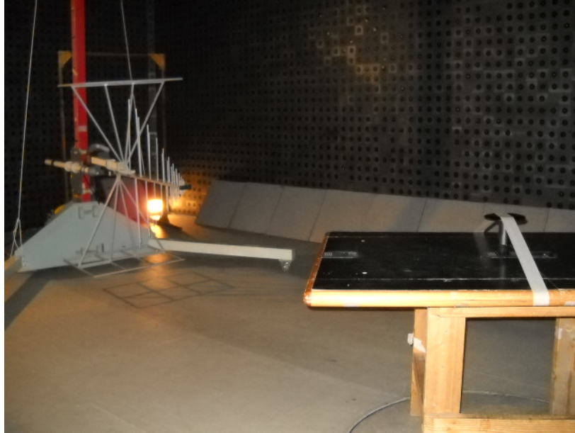
Photograph No.1 Setup for carrier field strength and power spectral density measurements in the anechoic chamber from 30 to 1000 MHz
