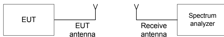
Figure 7.1.1 The 6 dB bandwidth test setup
