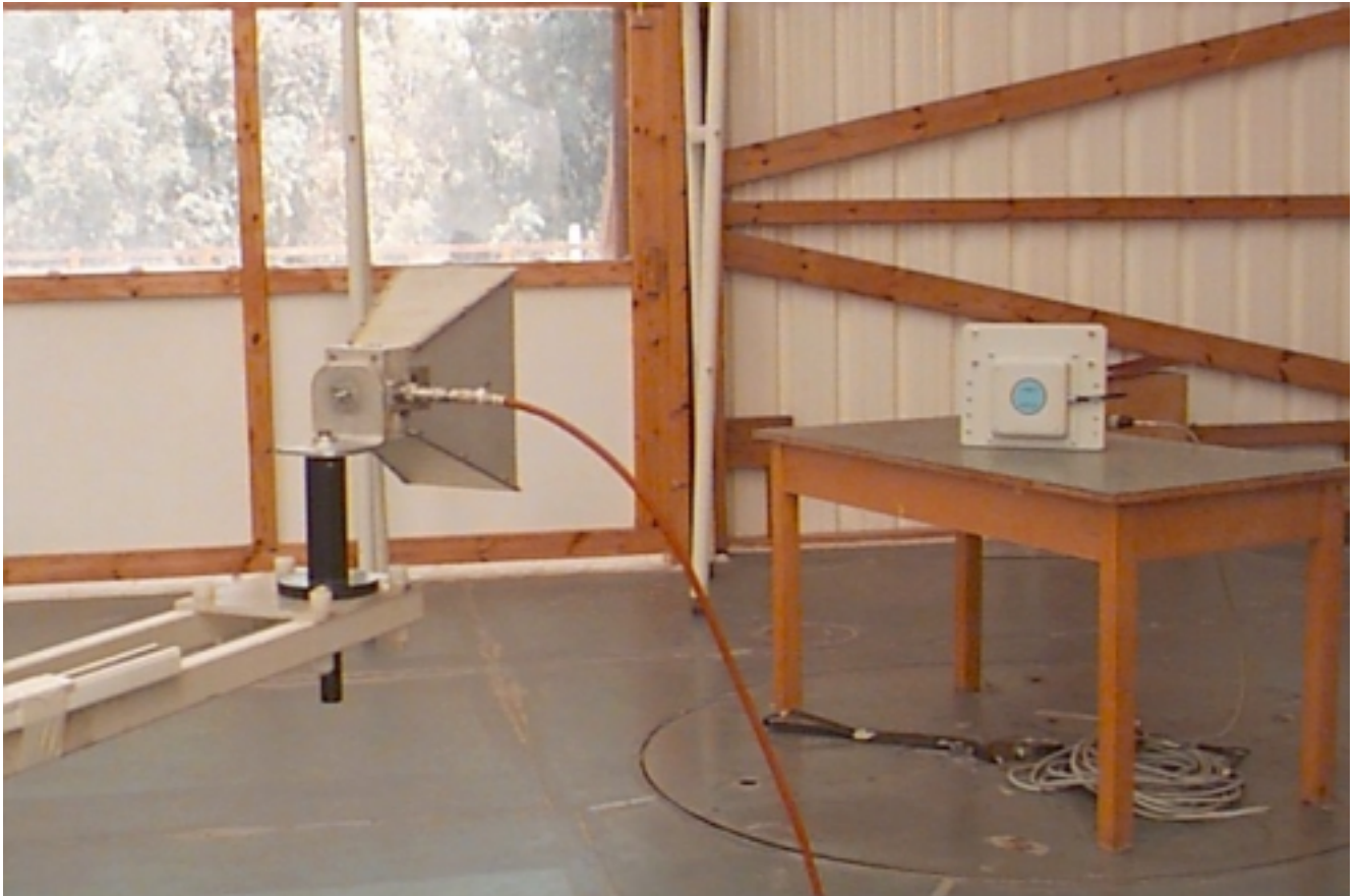
Photograph 4.6.1 Radiated emission measurement test setup
