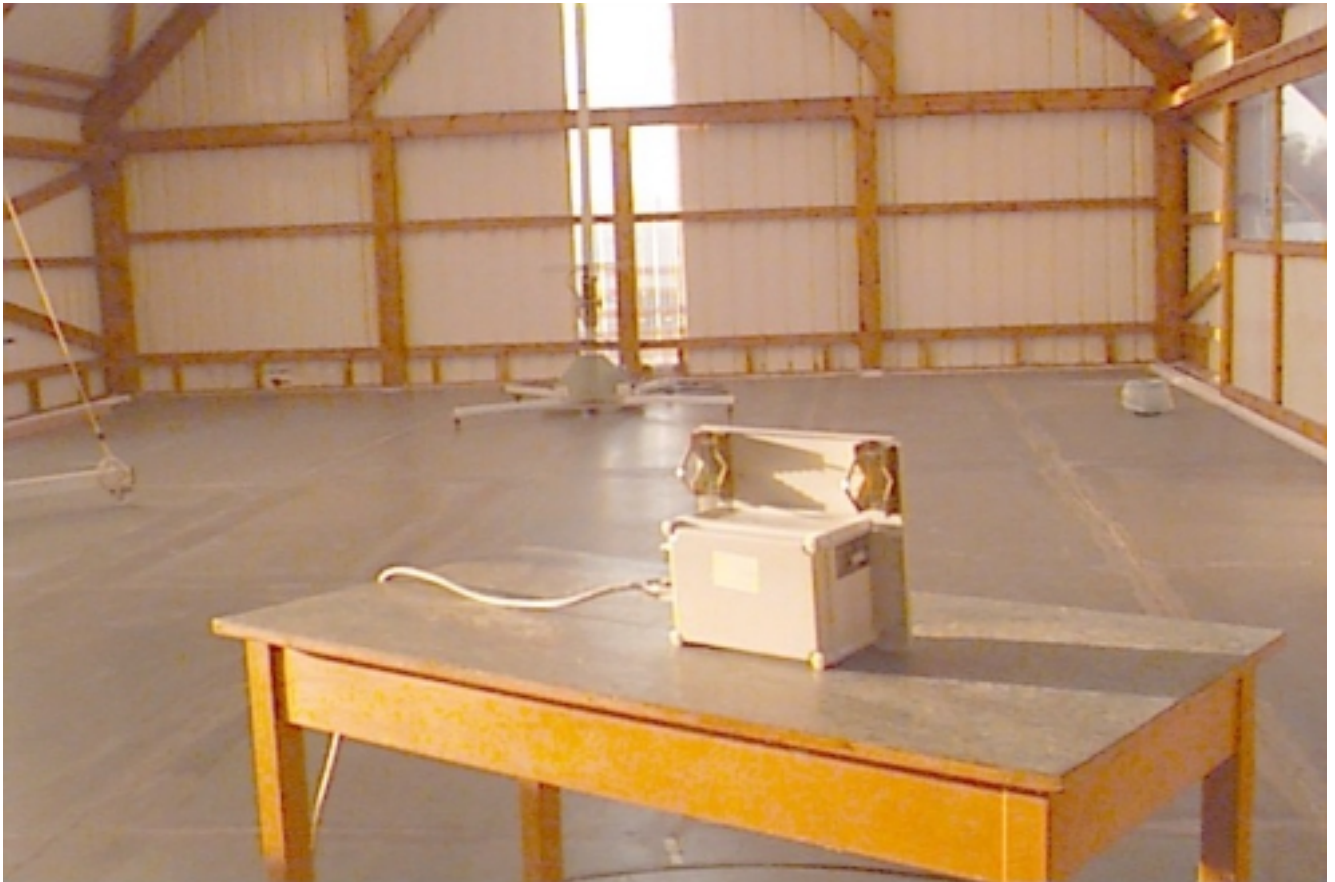
Photograph 4.8.1 Setup for radiated emission measurements
