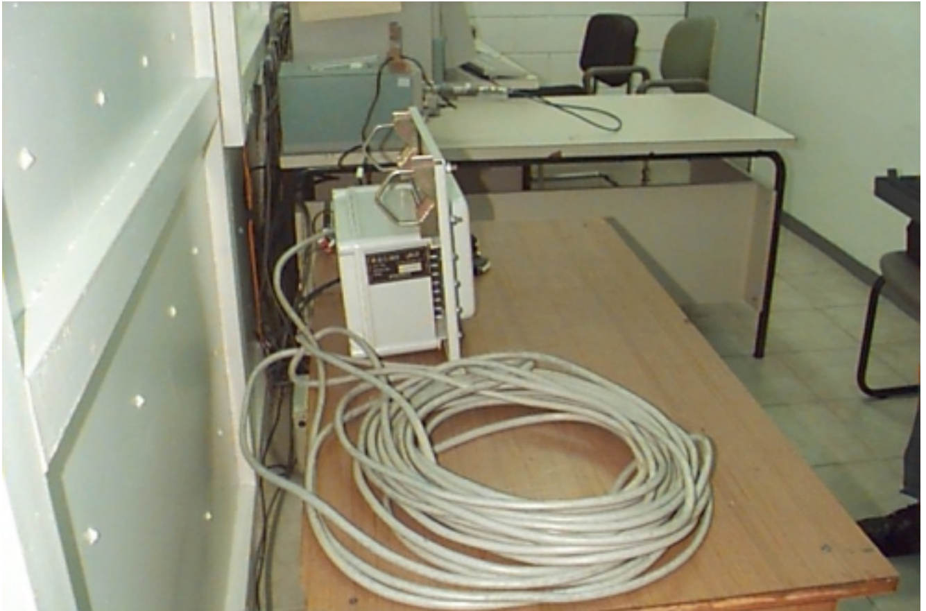
Photograph 4.7.2 Setup for conducted emission test
