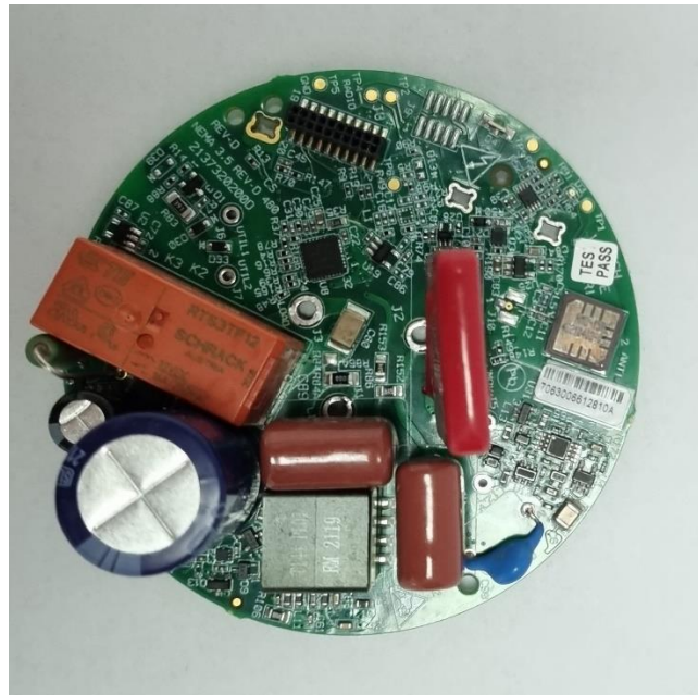
Platform (NEMA3.5) card- top view
