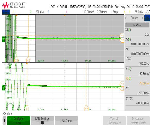
Plot 7.6.2 Transient frequency during power OFF test results at low carrier frequency
