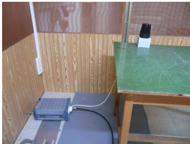
Photograph 7.6.1 Setup for conducted emission measurements
