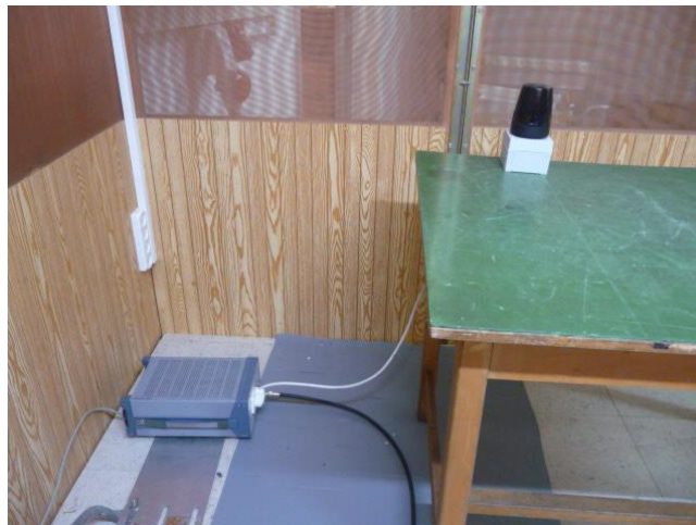
Photograph 8.1.1 Setup for conducted emission measurements
