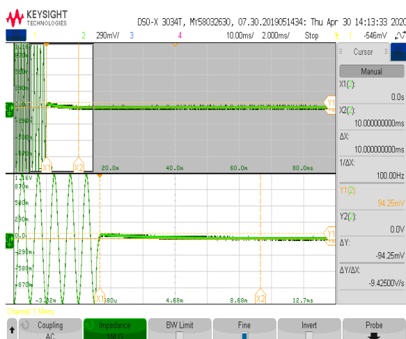
Plot 7.6.3 Transient frequency during power ON test results at mid carrier frequency
