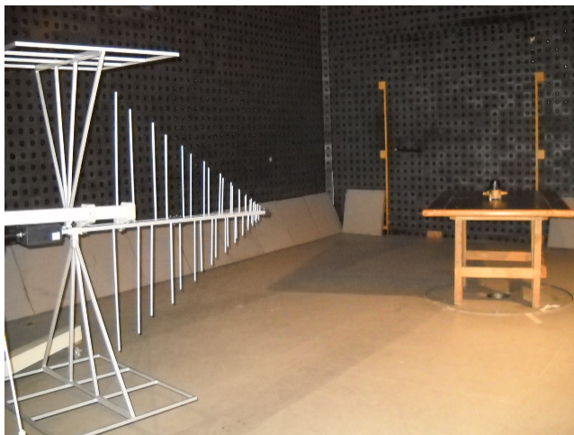
Photograph 8.1.1 Setup for radiated emission measurements, general view
