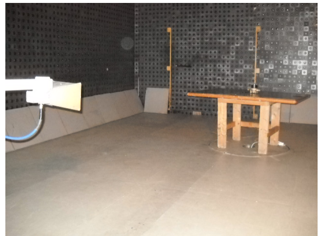
Photograph 8.1.1 Setup for radiated emission measurements, general view
