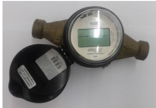
allegro internal antenna - top view
