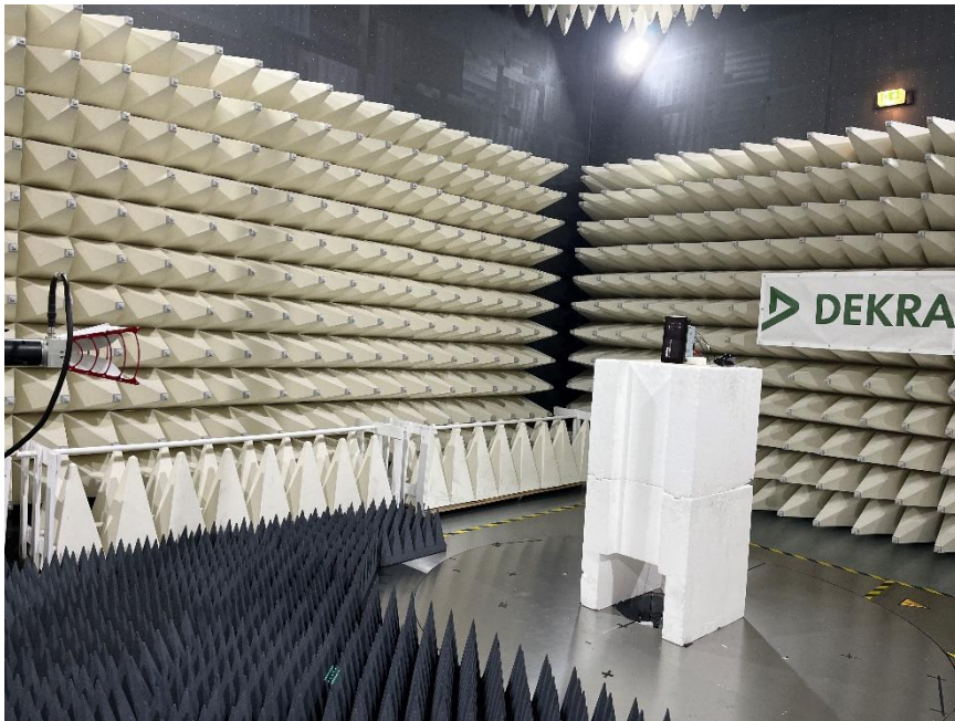
Figure B6. High Range Radiated Emission test setup 1-18GHz
