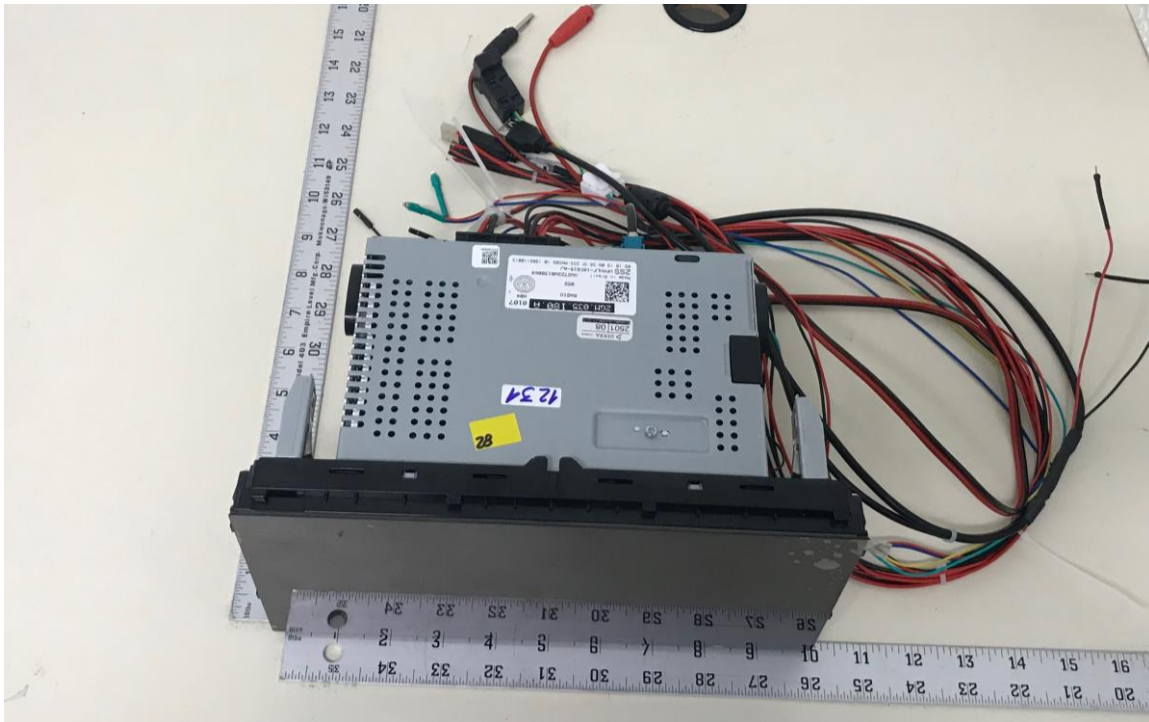
Figure C1: Conducted DUT Set up
