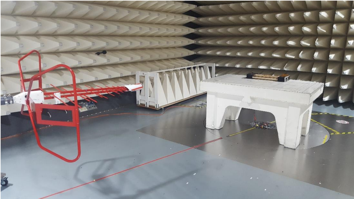
Figure B4. Radiated emission Setup – Low Range 30 to 1000 MHz
