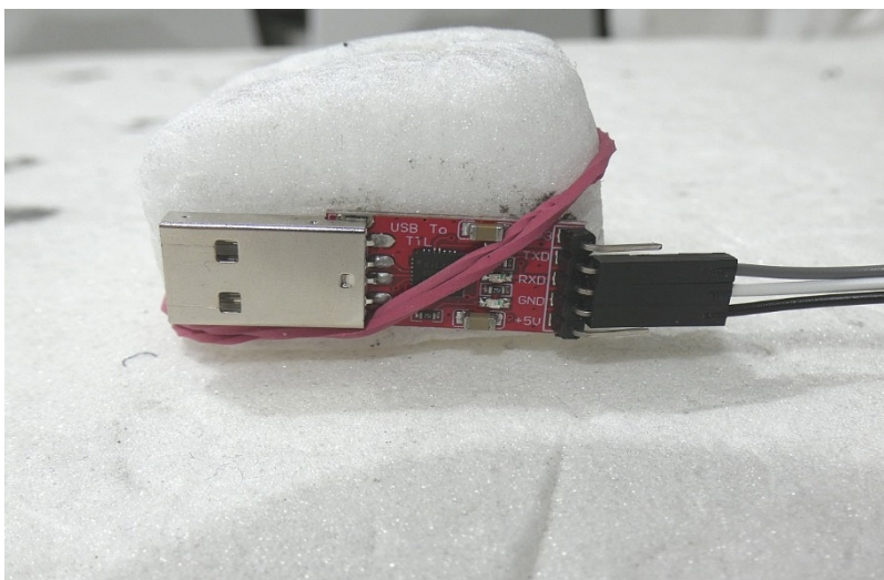
Photo 11: Auxiliary TTL-USB converter, detail
