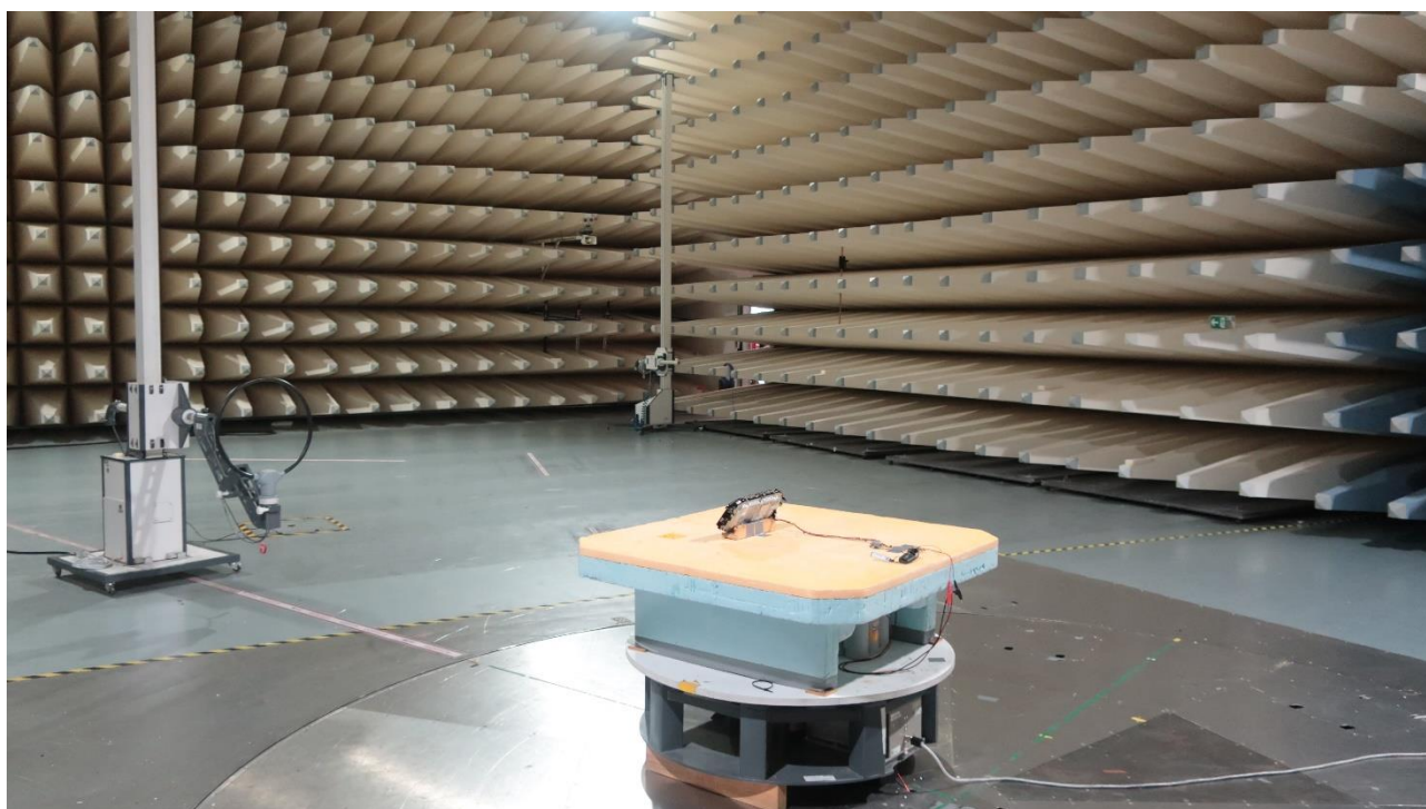
Photograph 2: Setup of radiated emissions measurement in the frequency range 9 kHz – 30 MHz (rear)
