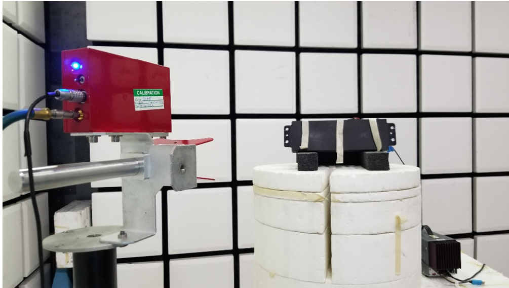
Photo 5: Emissions in frequency range 18-40 GHz
