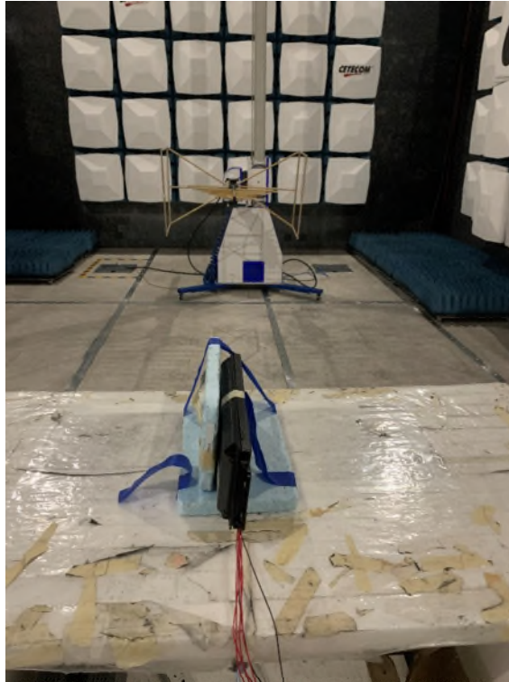
Photo 1: Emissions in frequency range 30 MHz to 1 GHz
