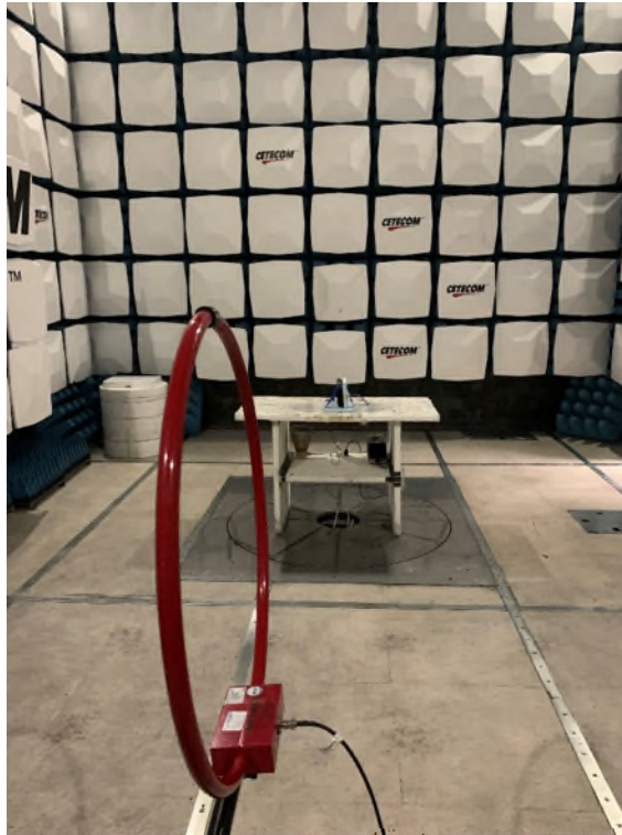
Photo 1: Emissions in frequency range 9 kHz to 30 MHz
