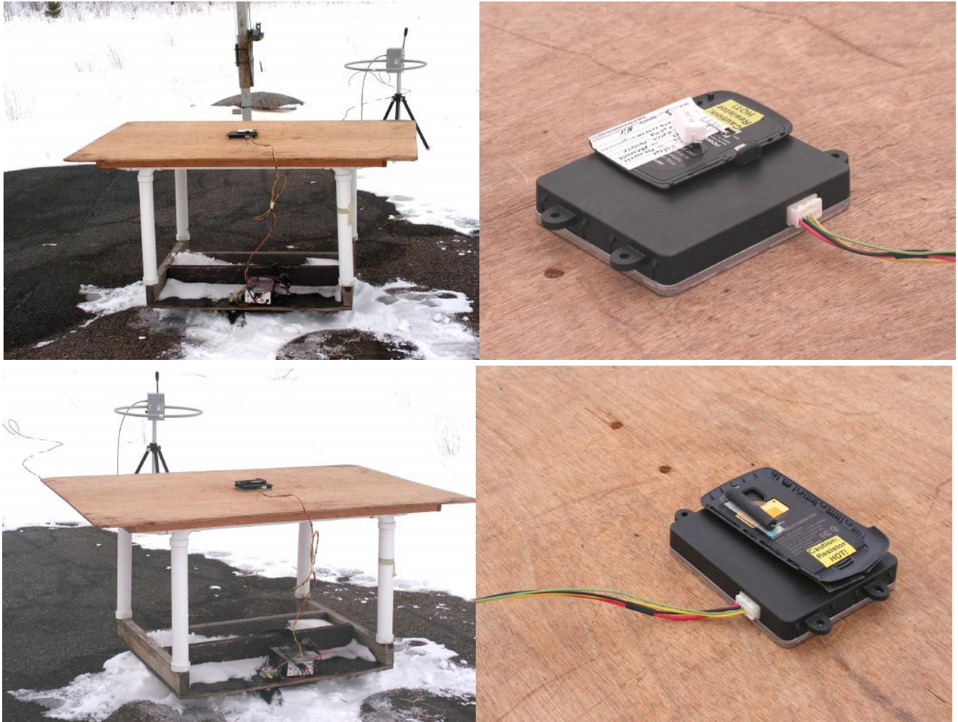
Figure 4: Radiated Emissions Test Setup Photograph(s).
