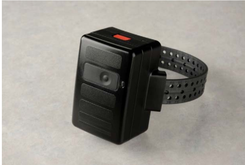
Figure 2: GPS device clipped on to body-worn PID3 device
