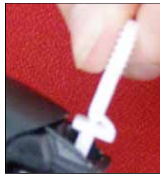
Figure 16: Proper Orientation of Retaining Pin
