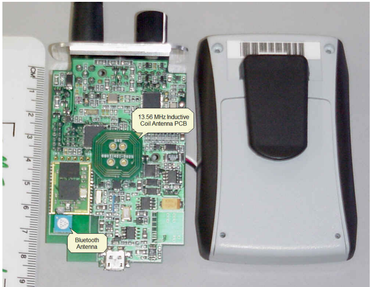
Figure 4: Top view of main PCB showing location of various antenna's (scale in centimeters is included for measurement reference purposes)
