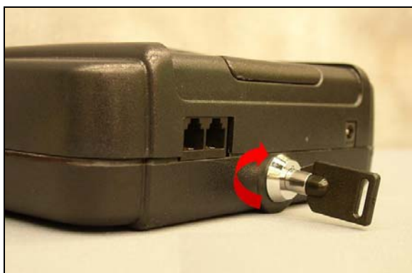
Figure 21: Turning PHMU Menu Key
