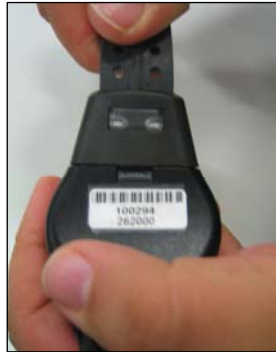
Figure 18: Window for viewing PTX Retaining Pin
