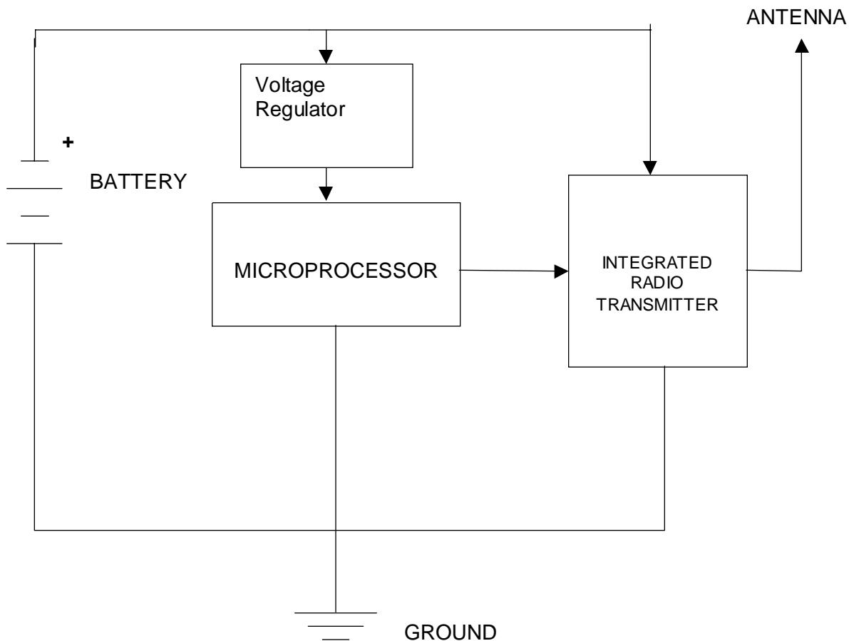
**NOTE: EUT TESTED WITH A FULL CAPACITY BATTERY TO DEMONSTRATE THE HIGHEST RF LEVEL AVAILABLE SINCE RF MODULE HAS NO VOLTAGE REGULATION.**
