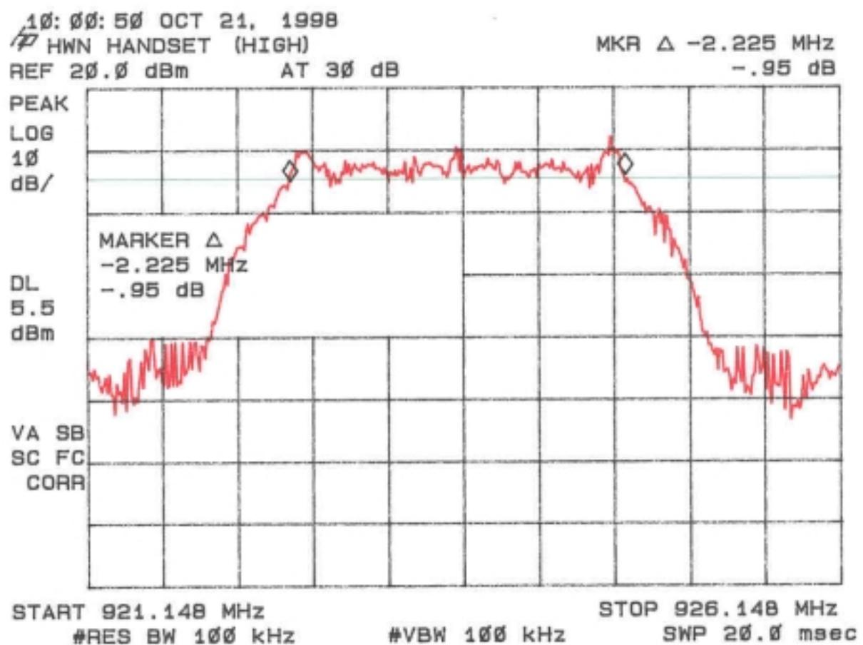
**2.11 Power Spectral Density FCC Section 15.247(b) and 15.247(d)**
