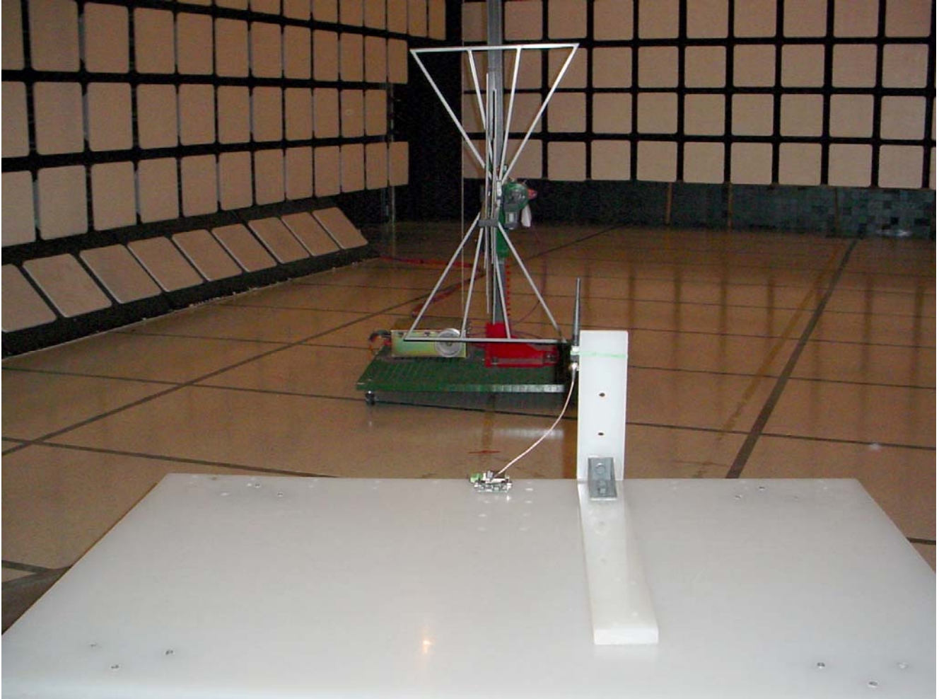
Radiated Emissions @ 3 m EUT with 2 dBi Rubber Ducky Antenna
