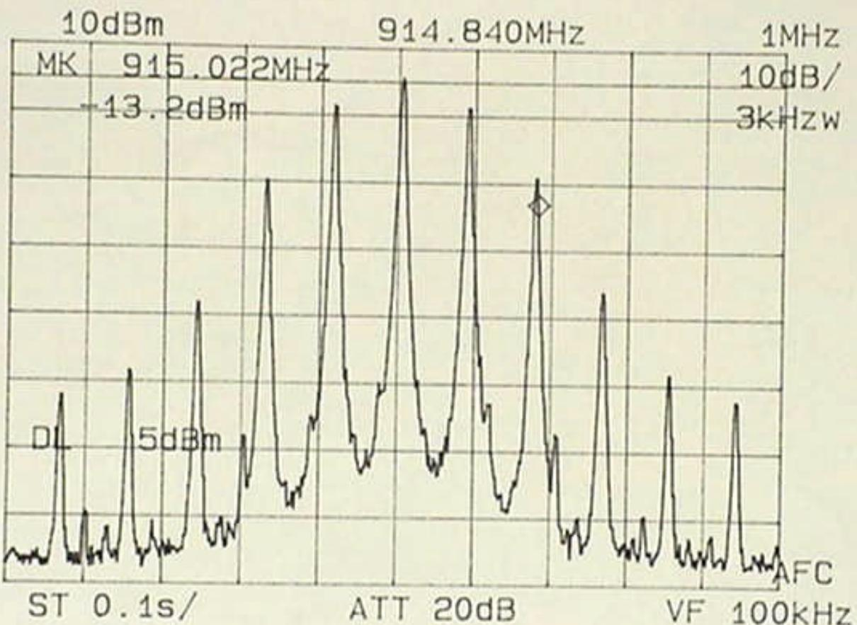
**4.2.3 20 dB Bandwidth Emissions (3 kHz Res. BW) High Channel Bandwidth Plot:**
