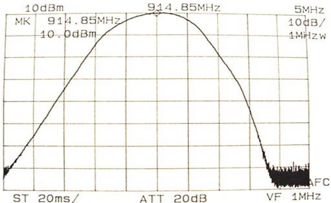
**4.1.3 Peak Power Modulated Carrier (1 MHz Res. BW) High Channel Plot:**
