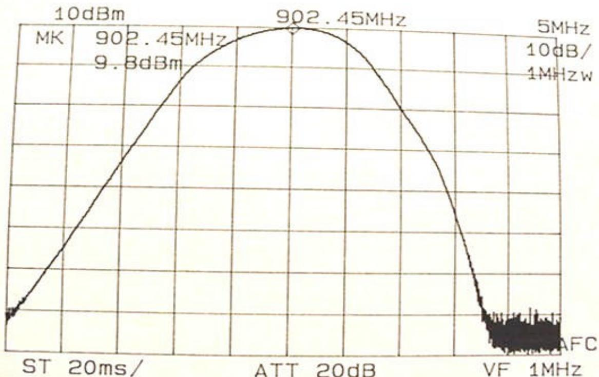
**4.1.2 Peak Power Modulated Carrier (1 MHz Res. BW) Mid Channel Plot:**
