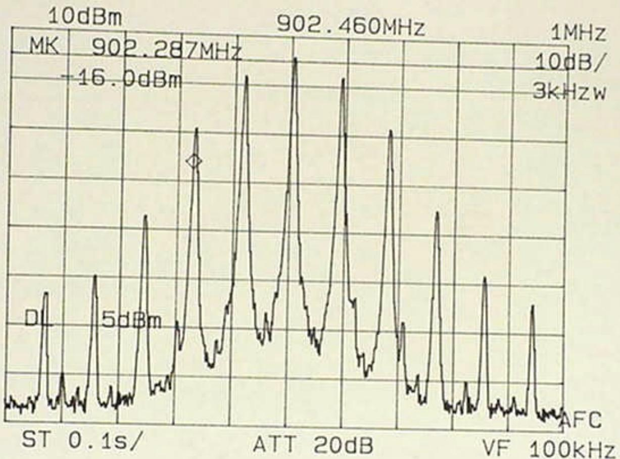
**4.2.2 20 dB Bandwidth Emissions (3 kHz Res. BW) Mid Channel Bandwidth Plot:**
