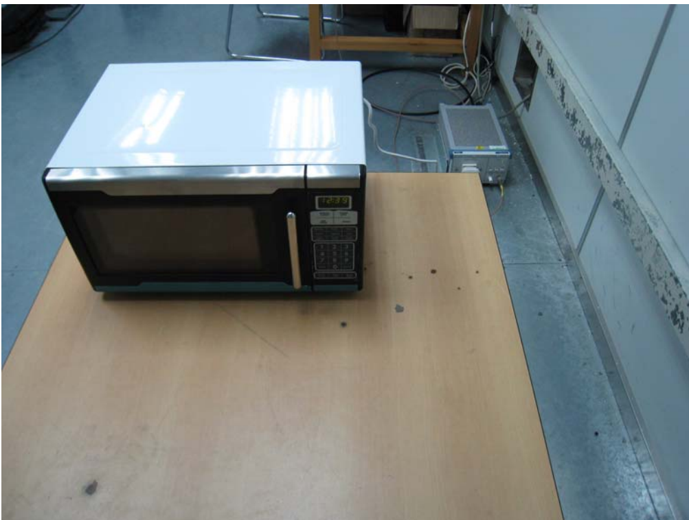
Photo 4 Conducted Disturbance Test (MEW622-A)
