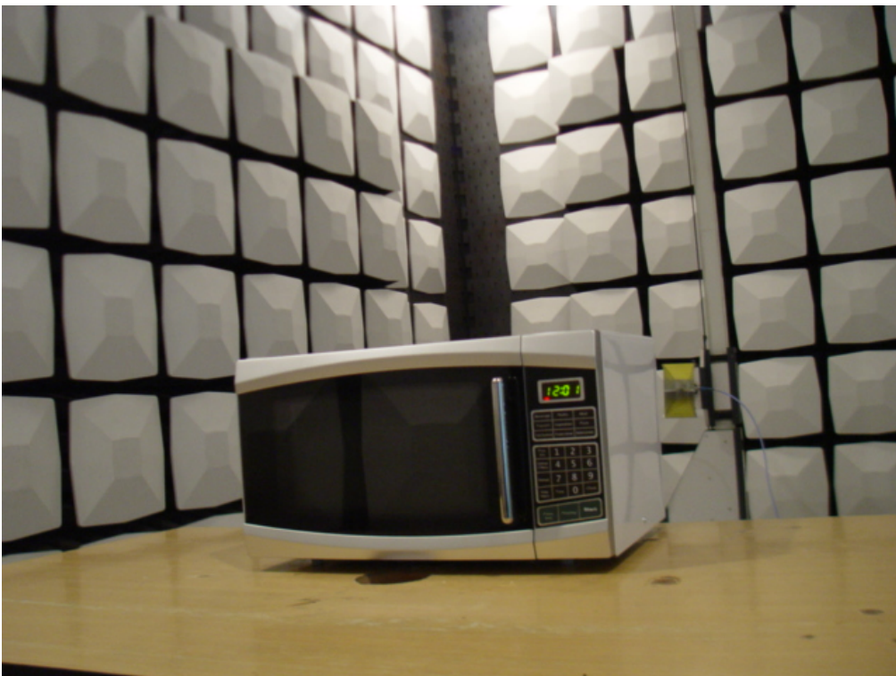
Photo 6 Radiated Disturbance Test (above 1GHz) (MEW621-A)
