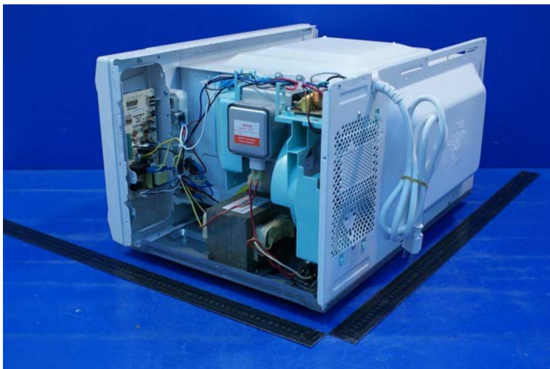
Photo 3 Internal photo of EUT (MEW621-A)
