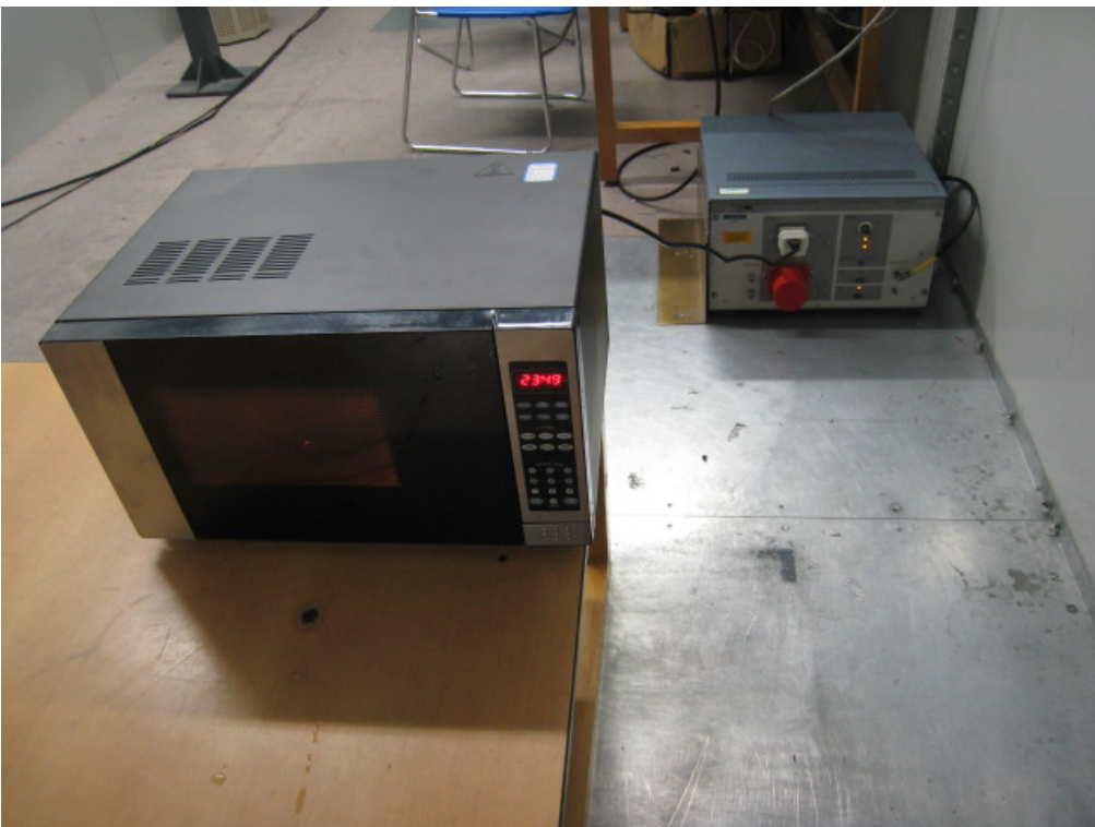
Photo 2 Conducted Disturbance Test (MEW60A-A)
