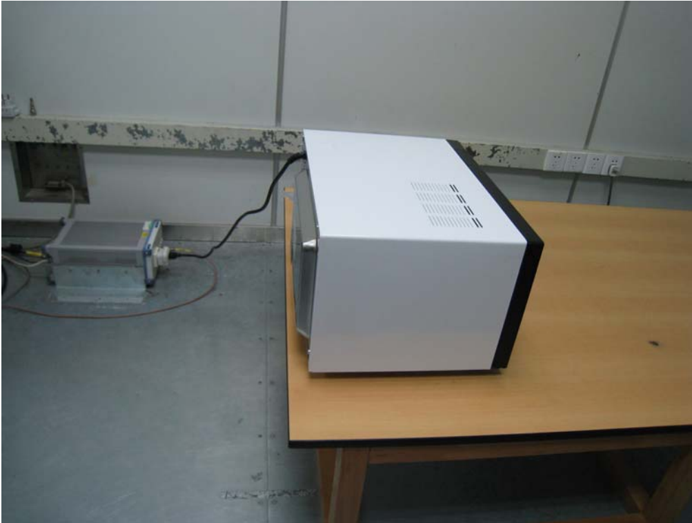
Photo 4 Conducted Disturbance Test (MEW60A-A)
