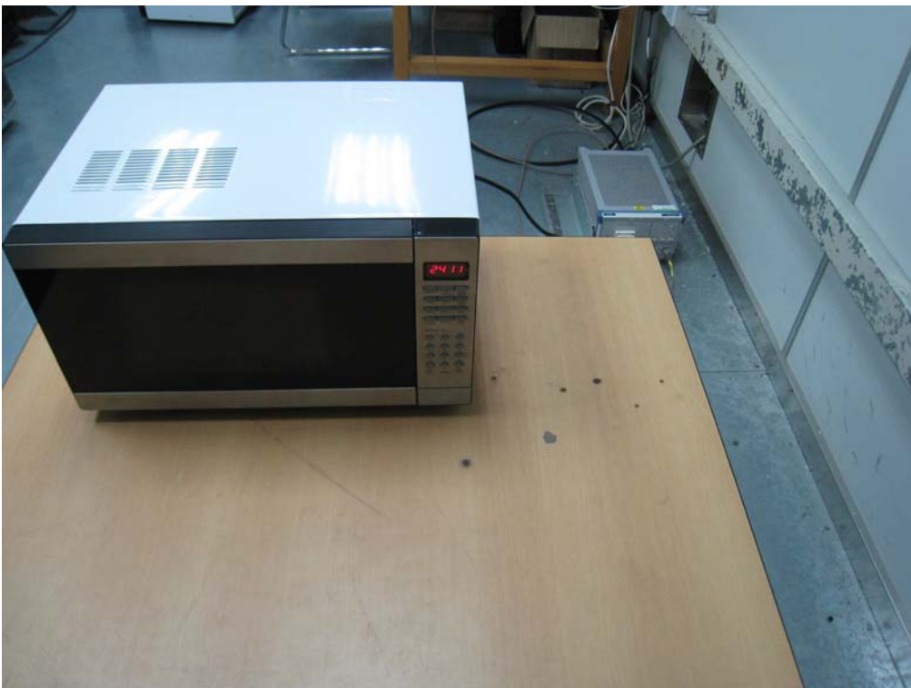
Photo 4 Conducted Disturbance Test (MEW60A-A)
