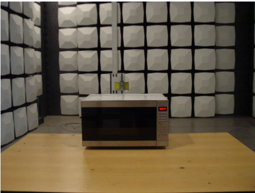
Photo 8 Radiated Disturbance Test (above 1GHz) (MEW60A-B)
